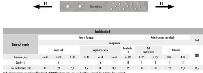
The load-bearing capacities were determined based on ETA-19/0020 Characteristic load-bearing capacity in kN, wood strength class 350 kg/m<sup>3</sup> char. Gross density. The minimum distances between the connectors and the edges according to EC5 must be complied with. Boundary bearing force according to EC3: Fa, R4 Ø14mm = 93, 75 kN
