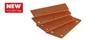
The Eurotec SonoTec Angular Decoupler forms the perfect complement to the Eurotec Shearing Angles and the CLT System Angle. The underlay is made from SK04, which is a compound formed from cork and natural rubber. The product is suitable for vibration damping applications in which very high insulation values are required. SonoTec angular decouplers are used as invisible insulators (pads/strips) with a low resonance frequency and a medium-low load.
