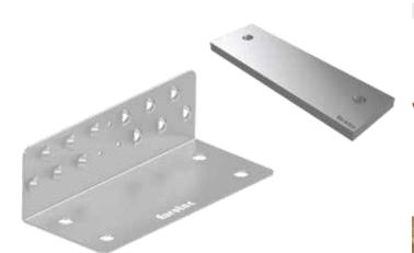
Art. no.Dimensions [mm]<sup>a)</sup>MaterialMaterial thickness [mm]954087100 x 230 x 70\$250 Galvanised3Shearing angle pressure plate954111230 x 68 x 12\$235 Galvanised3a) Length x height x depth\$235 Galvanised3
