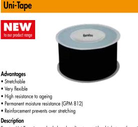
Eurotec Uni Tape is a polyethylene bonding tape with a high-strength, moisture-resistant polyacrylate adhesive with excellent ageing resistance. Designed for interior airtight bonding and sealing of vapour barrier and air-tight membrane overlaps and penetrations in accordance with DIN 4108-7. Uni Tape is also suitable for bonding polypropylene fleece material, aluminium sheeting, MDF and plywood panels as well as plastics.
