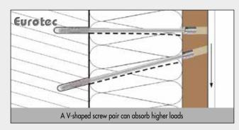
To increase the rigidity of the EiSYS-H system, the adjusting screws are installed in pairs and in a V shape. This creates a framework screw connection. The framework principle consists of creating a large number of rigid triangles (see diagram) from multiple relatively pliable screws installed perpendicular to the wall.
