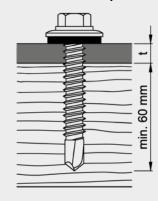
Steel on timber/timber on timber for BiGHTY bimetal 6,5 x L, drilling capacity 5 mm
