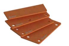
The Eurotec SonoTec Angular Decoupler forms the perfect complement to the Eurotec Shearing Angles and the CLT System Angle. The underlay is made from SK04, which is a compound formed from cork and natural rubber. The product is suitable for vibration damping applications in which very high insulation values are required. SonoTec angular decouplers are used as invisible insulators (pads/strips) with a low resonance frequency and a medium-low load.
