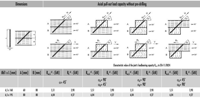
Calculation according to ETA-11/0024. Wood density px= 380 kg/m<sup>3</sup>. All mechanical values provided should be viewed as subject to the assumptions that have been made and represent example calculations.
