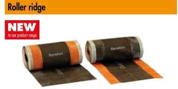
The roll ridge is made of high-quality, diffusible PP fleece (150 g) and pleated aluminium sheet. Thanks to the fleece, the tape enables ventilation between the eaves and the ridge. All without any risk of water or rodents getting underneath the roof structure.
